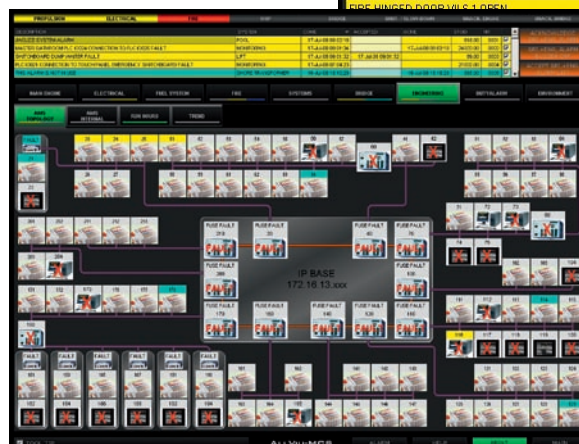
All relevant information is shown together with the network topology by besecke monitoring system.
