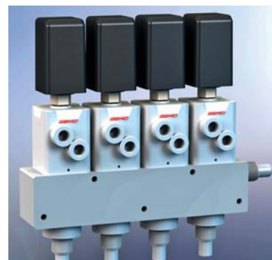
4-way block in PTFE with flare connections, pneumatic actuators type GEMÜ C50 and GEMÜ 1234 electrical position indicators
