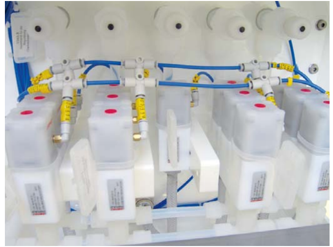
Block valve unit in production plant (Singulus Stangl Solar) for CIS cells
